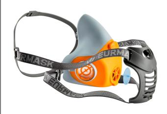
VULCANO is a one-size-fits-all half mask, in compliance with norm EN 140:1998, and in agreement with EU 2016/425 Regulation, with two quick bayonet connections for filters series 2000. Its ideal for the protection against both gross and fine dusts, inorganic/organic gases and vapours, acid gases and vapours, and combined gases and dusts.
